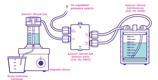
Amicon® Stirred Cell setup for large volume concentration and continuous diafiltration using selector valve and reservoir accessories.
