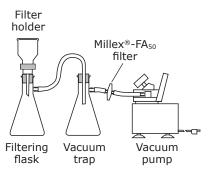
**NOTE:** For filter holders with stoppers, orient the longer side of the outlet spout towards the filtering flask sidearm, as shown.
