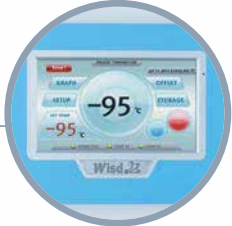
• Smart-Lab™ Controller - Easy setting, Temperature Graph, Storage function (USB interface), etc.
